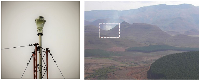
A typical camera used in ForestWatch CWDSs, and a fire detected by the system
